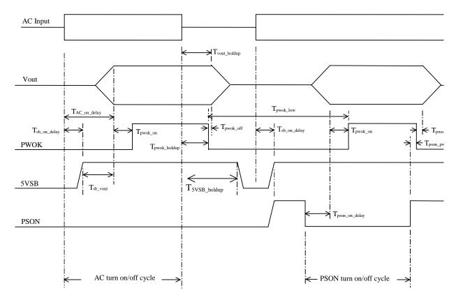
Figure 9. Turn On/Off Timing (Power Supply Signals)
